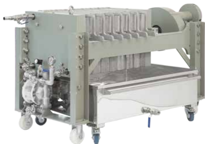
20" press 3 holes Filtration capacity: 15 to 50 barrels
