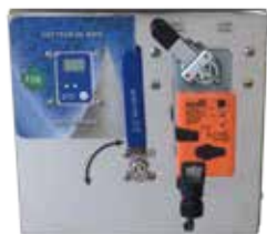
Continuous brix sensor with modulating valve
