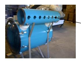
The wet and dry lines will come in the back of the manifold in the predrilled holes
