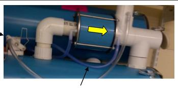
When the rocker arm is up, the vacuum is shifted from the left side of the cylinder to the right, through this tube
