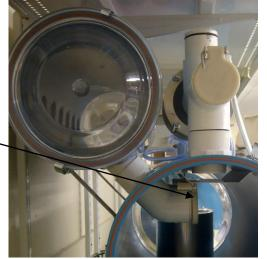
When the float gets to the bottom stopper, the weight of the float releases the rocker arm that goes down, shifts the cylinder to the left. This action allows vacuum to build again in the releaser, closing the bottom door, the cylinder cap and releasing the inside door
