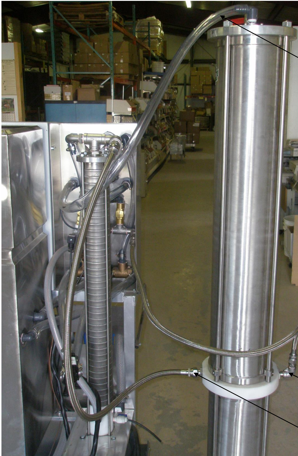
Hose hook up for a 600 GPH RO Picture 4
