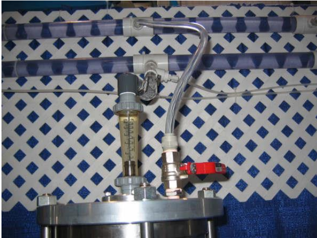
Top of RO post with optional individual flow meter
