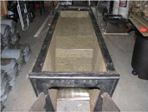
Insulating panels installed in the evaporator.
