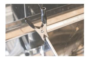
Connect 1/4 transparent tubing (EVAC-P00016) of probe to output of peristaltic pump. Tighten white nut.
