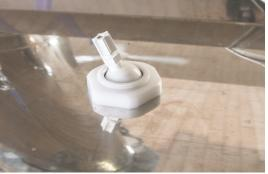
Unscrew 1/4 adapter nut so that the probe can be inserted into ball joint. Insert probe into the swivel until tip of stem is 2 inches lower than top of flue pan divider. Tighten white nut.
