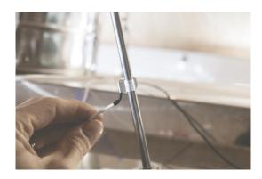
Make sure you have a 110 volt, grounded electrical outlet. Attach ground wire clamp (Ground) to float box.
