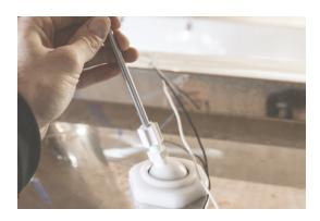
Attach probe wire (white wire) to the metal area of the probe.
