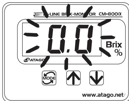
Fig.12-2 Example of the adjustment to the Brix 0.0%
