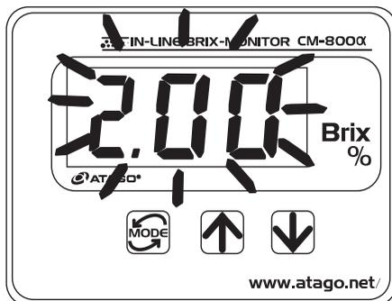
Fig.13-2 Example of the adjustment of the temperature correction factor to 2.00.
