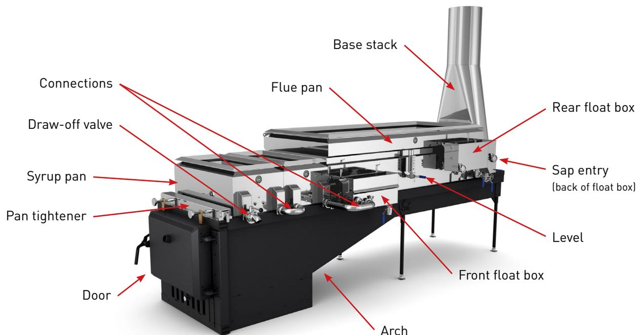
1. Set the pans on the evaporator starting with the flue pan. Make sure the back of the pan touches the back plate (or the reheat pan if you have one). Then, install the syrup pans in the front. Make sure the evaporator and the pan are leveled. Finally, tighten the pans together using the pan tightener.
