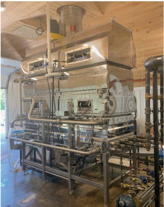
Picture: R7 system including pan washer, steam pan and high pressure plumbing options.
