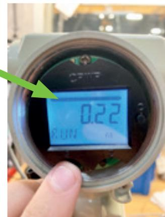
To set your low level, remove water until it reaches -3", then press and hold the S and Z buttons simultaneously for 15 seconds until "Z50K" appears. Once "Z50K" appears, release the buttons and press on the "Z" button (on the right) to record your low level. Afterwards, the black bar like the one in figure 3 will disappear (fig. 4). This means that your low level has been recorded.
