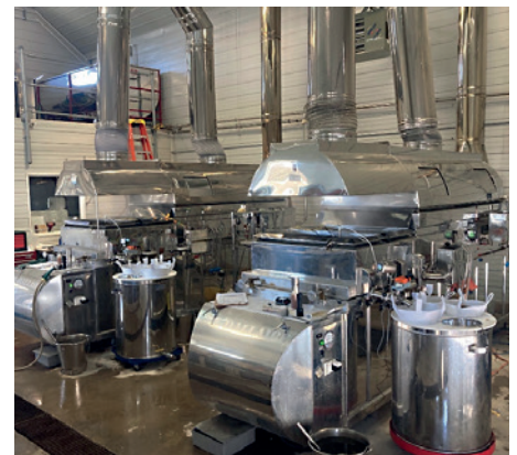
Maple Processing Research Facility at the University of Vermont Proctor Maple Research Center during an experiment processing pure red and sugar maple sap concentrated to 8%.
